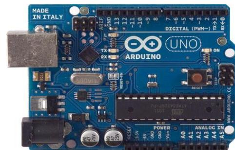
Gambar 2.9 Board Arduino Uno
